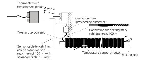
Depending on the internal temperature of EIGERFLEX®, the maximum length of the frost protection strip (without any additional power supply) is 50 to 100 m.
