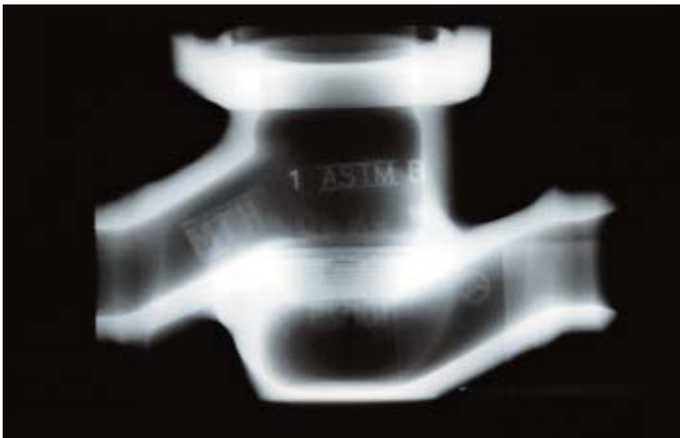
X-ray image of a cast-iron body with welded ends. Shrink holes and inclusions can only be detected with certainty in this way.
