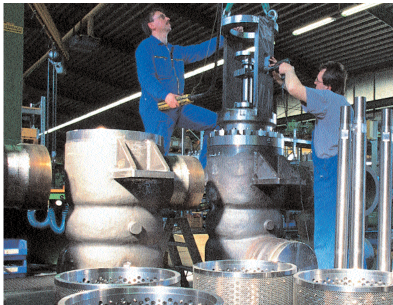
The assembly and testing of industrial valves, that weigh tons calls for millimetre precision and finger-tip feeling – as in these eight turbine bypass valves for a power plant in India. Complicated function tests and final approval testing over several days face the assembly personnel with ever new challenge.
