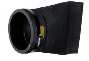
The valve consists of an elastomer 'duckbill' with a slip-on connection. This simple rugged design eliminates the mechanical parts which can wear and jam in conventional check valves.
