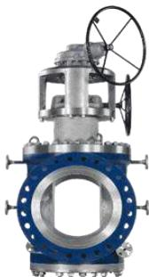
**SchuF** is the original inventor of the **Lift Plug Valve** designed to deliver 100% seal tightness with non-wearing internal movement and full-bore unimpeded flow in severe applications. It's simple, gasket-free design minimizes maintenance and prevents clogging.
