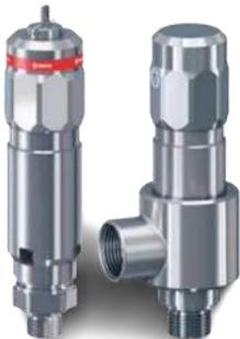
**Goetze High Pressure Safety Valves** can be used in industrial gas applications up to 21,756 psi and are installed in hydrogen refueling stations around the world. Goetze also manufactures **pressure reducing valves** for gas regulation with a cartridge design for easy servicing without valve removal.
