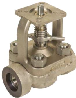
Reduce maintenance costs and downtime with the **Conval Camseal Ball Valve**. The top-entry design enables in-line renewal and zero leakage restoration in just 30 minutes! Type-tested with high-pressure nitrogen, it achieved zero bubbles in four minutes—proof of superior sealing and durability.
